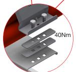
To assure a secure fit of the cable(s), a clearance greater than zero and less than the thickness of one shim-plate is recommended. One additional pair of shim plates is needed if the clearance is larger than the thickness of one shim plate (2.5mm).
