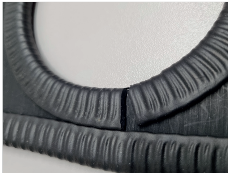
Individual SS legs are encapsulated in EPDM rubber
