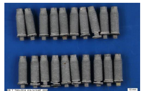
Removed S-BT HL fastenings after 12 weeks EN ISO 16701 cyclic corrosion test. No visible corrosion.
