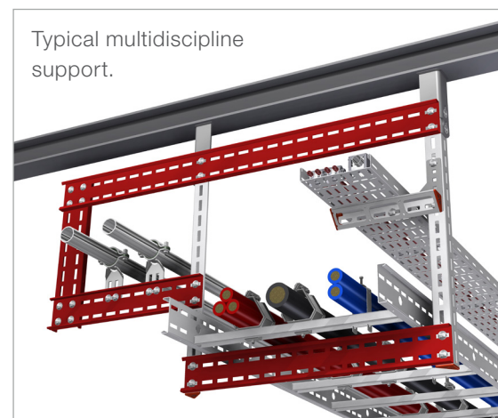
CH100-1 fitted directly to support
