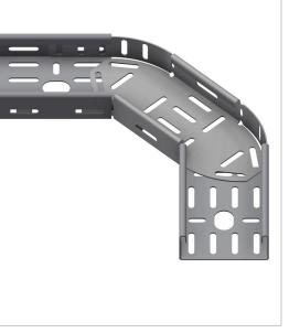
SPB-RF Flexi Elbow Covers suit all angles. The cover from connecting cable tray is fitted over the Flexi Elbow Cover. Use 3 clamps from width 300 mm and over. Use Hurricane clamp where high wind loadings can occur.
