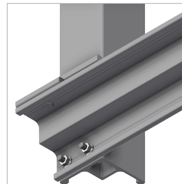
Vertical channel to horizontal channel joint detail (bottom view).
